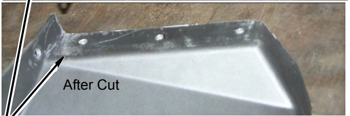
Mounting Tab Cut (before and after)
